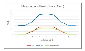
Fig. 4. Measurement Result (Power)
