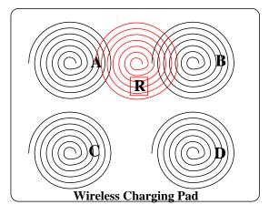
Fig. 6. Scenario 2 one-by-two coil (Worse)
