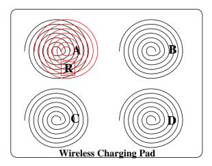
Fig. 5. Scenario 1 one-by-one coil (Good)
